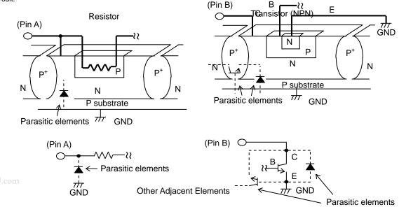
Simplified structure of a Monolithic IC
